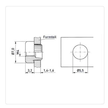
Finish: Plain Height [mm]: 3.2 Material: Steel Material Group: Steel Outer Diameter [mm]: 7 Panel Hole Ø [mm]: 5.5 Panel Thickness [mm]: 1,4 - 1,6 Thread Size: M4 Weight: 0.76g
