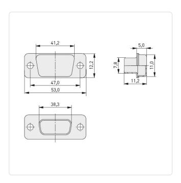
Material: Steel Stahl Material Group: Model: D-Sub Mounting Hole [mm]: 3.2 Width [mm]: 53 Weight: 5.4g
