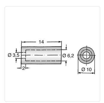
Color: Black Flammability Class: UL94-HB For Thread Size: M3.5 Inner Diameter [mm]: 6.2
