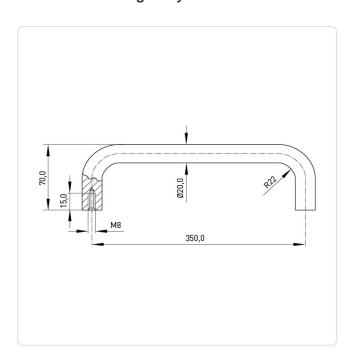
Dist. Mounting Holes [mm]: 350 Height [mm]: 70 Material: Steel Material Group: Stahl
