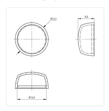
Color: Gray Head Height [mm]: 8 Inner Diameter [mm]: 12.8 Material: PA 6.0 Material Group: **Plastic**
