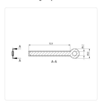
Color: Black Height [mm]: 52 Material: Steel Material Group: Steel Screw-On Model:
