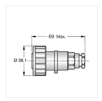
Amperage [A]: Color: Black Protection Code: IP68 Weight: 37g Conformities:
