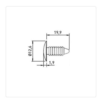
Color: Black Flammability Class: UL94-V2 Head Diameter [mm]: 12.6 Head Height [mm]: 1.9 Length [mm]: 19.9 Material: PA 6.6 Material Group: Plastic Mounting Hole [mm]: 6.4 Panel Thickness [mm]: 3,8-13,6 Weight: 0.61g
