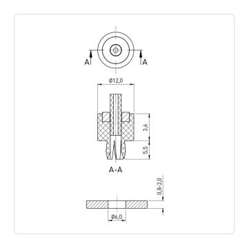
Color: Black Diameter [mm]: 12 Height [mm]: 3.6 Material: PA 6.0 Material Group: **Plastic** Panel Hole Ø [mm]: Panel Thickness [mm]: 0,8-2,0
