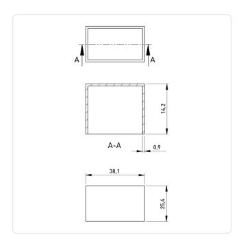
Color: Black Flammability Class: UL94-V0 Height [mm]: 14.2 Length [mm]: 38.1
