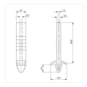
Color: Natural Flammability Class: UL94-V2 Length [mm]: 50.8 Material: PA 6.6 Plastic Material Group: Model: Plug-In Foot
