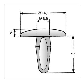
Color: Black Flammability Class: UL94-V2 Head Diameter [mm]: 14.1 PA 6.0 Material: Material Group: **Plastic**
