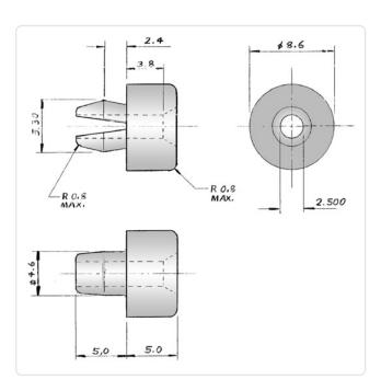
AF / OD [mm]: 8.6 Color: Natural Head Height [mm]: 5 Length [mm]: 5 PA 6.6 Material: Material Group: Plastic Panel Cutout [mm]: 4.6x4.6 Panel Thickness [mm]: 0,8-2,0 Thread Diameter [mm]: Ø 3.5 Weight: 0.4g Conformities:
