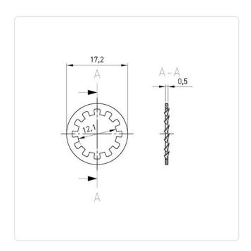
Finish: Alkaline Galvanized 8 µm
