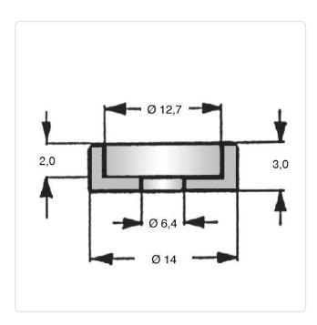
Color: Black For Thread Size: M6 Height [mm]: Inner Diameter [mm]: 6.4 Material: PA 6.0 Material Group: Plastic Outer Diameter [mm]: 14 Weight: 0.2g
