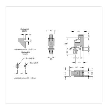
Color: Natural Flammability Class: UL94-V2 22.1 Length [mm]: PA 6.6 Material: Material Group: **Plastic** PCB Thickness [mm]: 1,6-2,3 Panel Hole Ø [mm]: 4.8 Panel Thickness [mm]: 1,0-2,3 Weight: 1.1g
