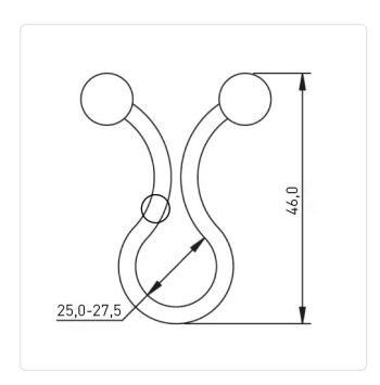
Bundle Diameter [mm]: 25,0-30,0 Color: Natural Flammability Class: UL94-V2 Material: PA 6.6 Material Group: **Plastic** Weight: 0.83g
