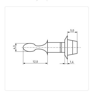
Color: Natural PA 6.6 Material: Material Group: Plastic Thread 1 Length [mm]: 12 Width [mm]: 4.3 Weight: 0.73g Conformities:
