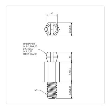
Color: Natural UL94-V2 Flammability Class: 4.8 Length [mm]: PA 6.6 Material: Material Group: **Plastic** PCB Hole Ø [mm]: 3.9 PCB Thickness [mm]: 1,6 Thread Size: М3 Weight: 0.18g
