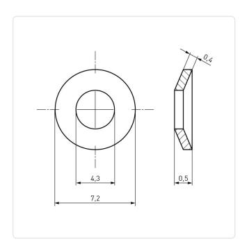
Finish: Plain For Thread Size: M4 Height [mm]: 0.4 Inner Diameter [mm]: 4.3
