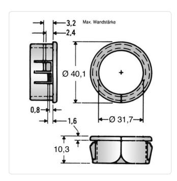
Color: Black Inner Diameter [mm]: 31.7 Material: PA 6.6 Plastic Material Group: Max. Panel Thickness [mm]: 3.2 Mounting Hole [mm]: 38.1 Outer Diameter [mm]: 40.1 Weight: 2.8g
