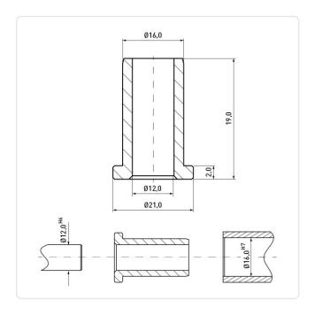
Color: Natural Flammability Class: UL94-V2 Inner Diameter [mm]: 12
