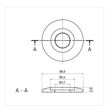
Finish: Nickel-Plated, 3 µm, E1E Brass CW614N / CuZn39Pb3 Material:
