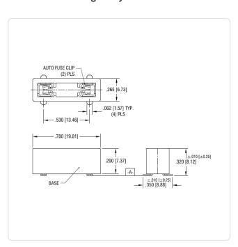
Amperage [A]: Fuse Size [mm]: 5.2x0.64 Material: **Brass** Material Group: Brass Model: Fuse Holder
