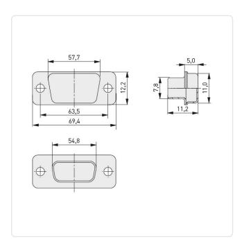
Material: Steel Stahl Material Group: Model: D-Sub Mounting Hole [mm]: 3.2 Width [mm]: 69.4 Weight: 7.38g
