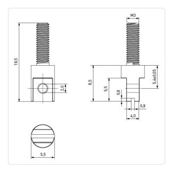
AF / OD [mm]: 5.5 Finish: Nickel-Plated, 3 µm, E1E Length [mm]: 8.5 Brass CW614N / CuZn39Pb3 Material: Material Group: Brass Thread 1 / Hole 1: М3 Thread 1 Length [mm]: 10 Thread 2 / Hole 2: Ø 2,0 Thread 2 Length [mm]: 4 Weight: 1.85g Conformities: Reach RoHS
