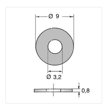
Color: Natural For Thread Size: МЗ Height [mm]: 8.0 Inner Diameter [mm]: 3.2 Material: PA 6.0 Material Group: Plastic Outer Diameter [mm]: 9 0.05g
