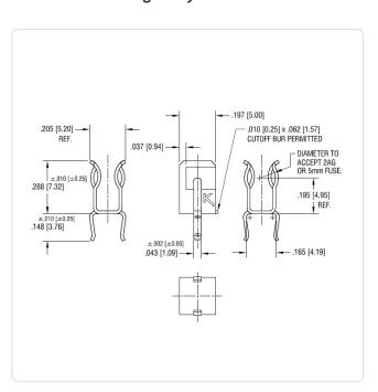
Fuse Size [mm]: 5.0x20.0 Material: Brass Material Group: **Brass** Model: Clip Holder
