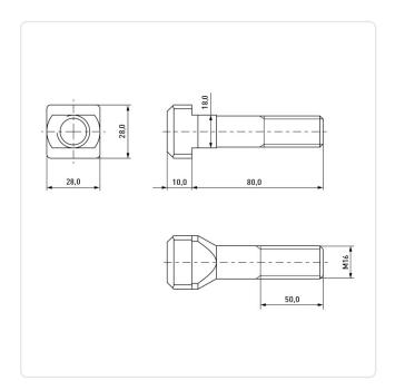
DIN/ISO: **DIN787** Plain Finish: Head Height [mm]:
