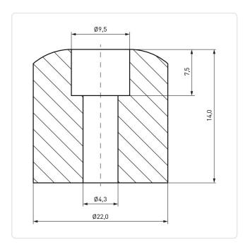
Bumper Design: Round Color: White Diameter [mm]: 22 Height [mm]: 14
