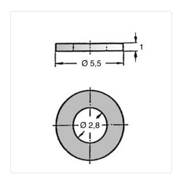
Color: Russet For Thread Size: МЗ Height [mm]: Inner Diameter [mm]: 2.8
