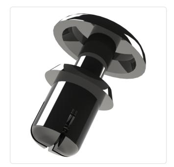
Color: Black UL94-V2 Flammability Class: Head Diameter [mm]: 7.8 Head Height [mm]: 1.9 Length [mm]: 6.1 Material: PA 6.6 Material Group: Plastic Model: removable Mounting Hole Range [mm]: Ø 4.1-4.2
