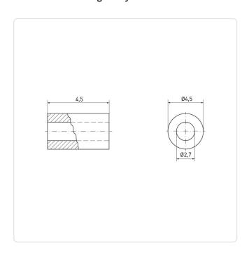
Finish: Plain For Thread Size: M2.5 Inner Diameter [mm]: 2.7 Length [mm]: 4.5
