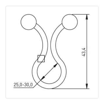
Bundle Diameter [mm]: 25,0-30,0 Color: Natural Flammability Class: UL94-V2 Material: PA 6.6 Plastic Material Group: Weight: 0.26g
