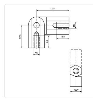
Finish: Nickel-Plated, 3 µm, E1E Leg Length 1 [mm]: 12.5 Leg Length 2 [mm]: 12.5 Length [mm]: 25 Material: Brass Material Group: Brass Model: Female/Female M4 Thread 1 Size: Thread 2 Size: M4 Weight: 6.8g Conformities: Reach RoHS SVHC
