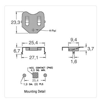
Battery Type: Cell Dia. 24mm
