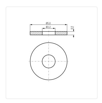
Color: Natural For Thread Size: M2 Height [mm]: 0.5 Inner Diameter [mm]: 2.2 Material: PA 6.0 Material Group: Plastic Outer Diameter [mm]: 5
