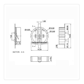
Battery Type: Cell Dia. 12mm
