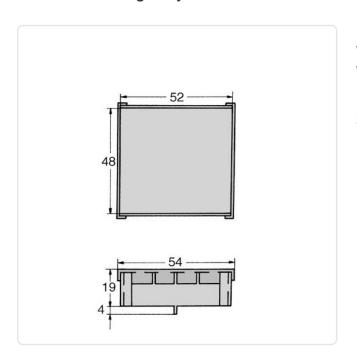
Height [mm]: 19 Length [mm]: 54 Material: Steel Material Group: Steel
