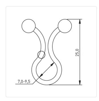
Bundle Diameter [mm]: 3,0-10,0 Color: Natural Flammability Class: UL94-V2 Material: PA 6.6 Plastic Material Group: Weight: 0.36g
