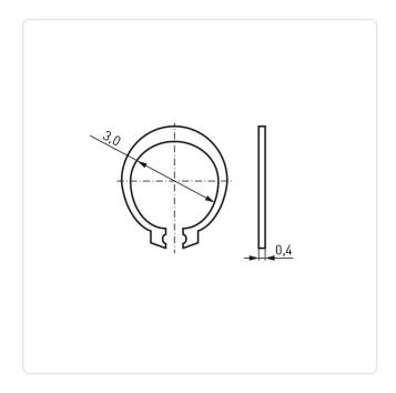
DIN/ISO: **DIN471** Finish: Plain 0.4 Height [mm]: Inner Diameter [mm]: 3
