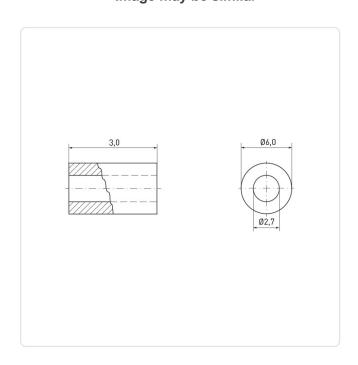
Color: Natural Flammability Class: UL94-HB For Thread Size: M2.5 Inner Diameter [mm]: 2.7 Length [mm]:
